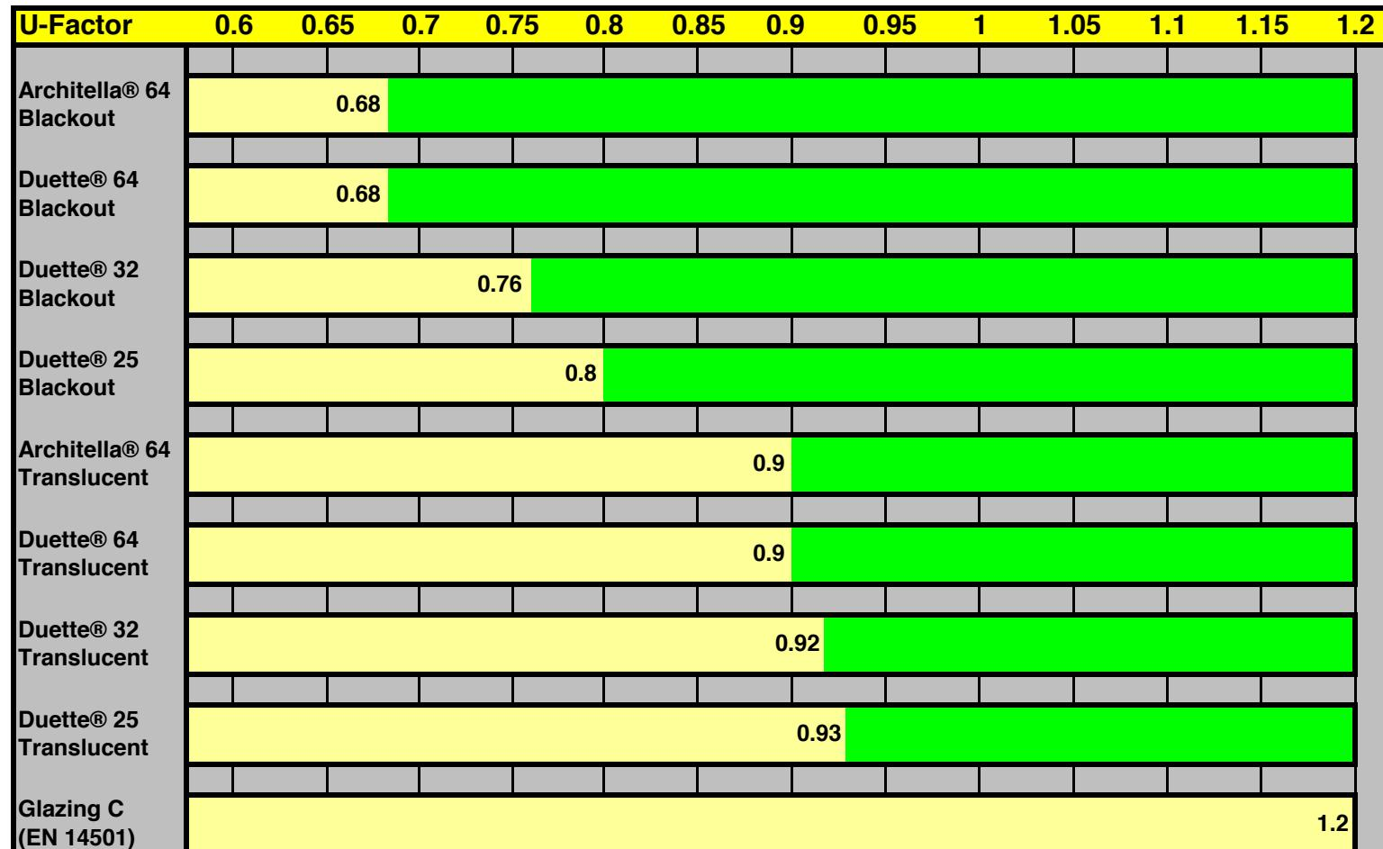
U-factors represent the combined total of the product's U-Factor and the U-Factor of Glazing C (according to EN14501).
